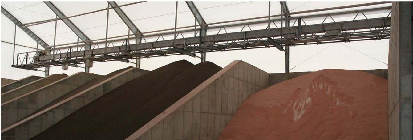
Figure III: Conveyor system for commodity and fertilizer storage
